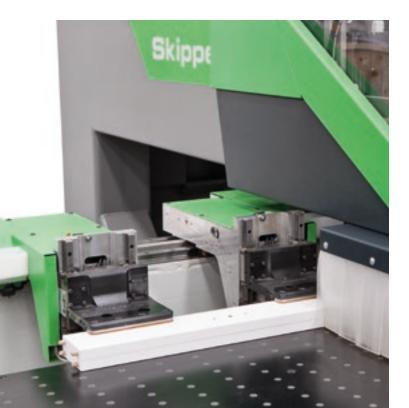
Skipper can easily perform "through" operations without any risk of splintering the material. It also processes "breathable" materials and very small pieces perfectly.
