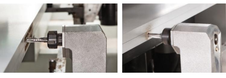
THE MACHINE CAN BE FITTED WITH ONE OR TWO INDEPENDENT HORIZONTAL UNITS.
