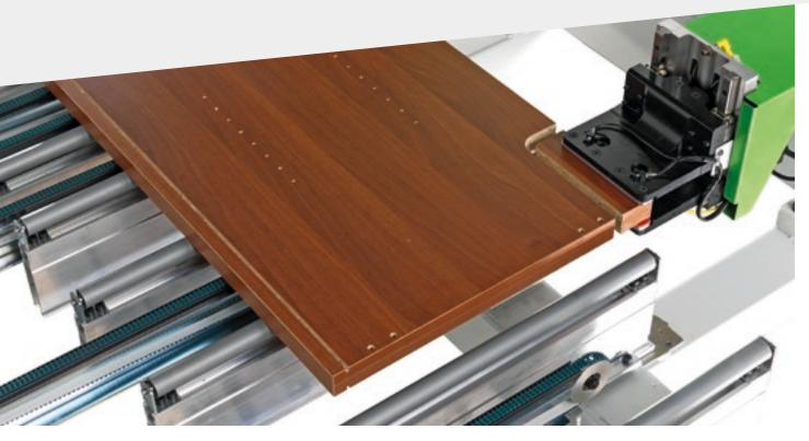
Complete flexibility for machining panels of different thicknesses and sizes. Simultaneous, continuous machining operations on both the upper part and the lower part, without the need to feed the panels through the machine several times.
